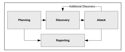
Figure 5-1. Four-Stage Penetration Testing Methodology
